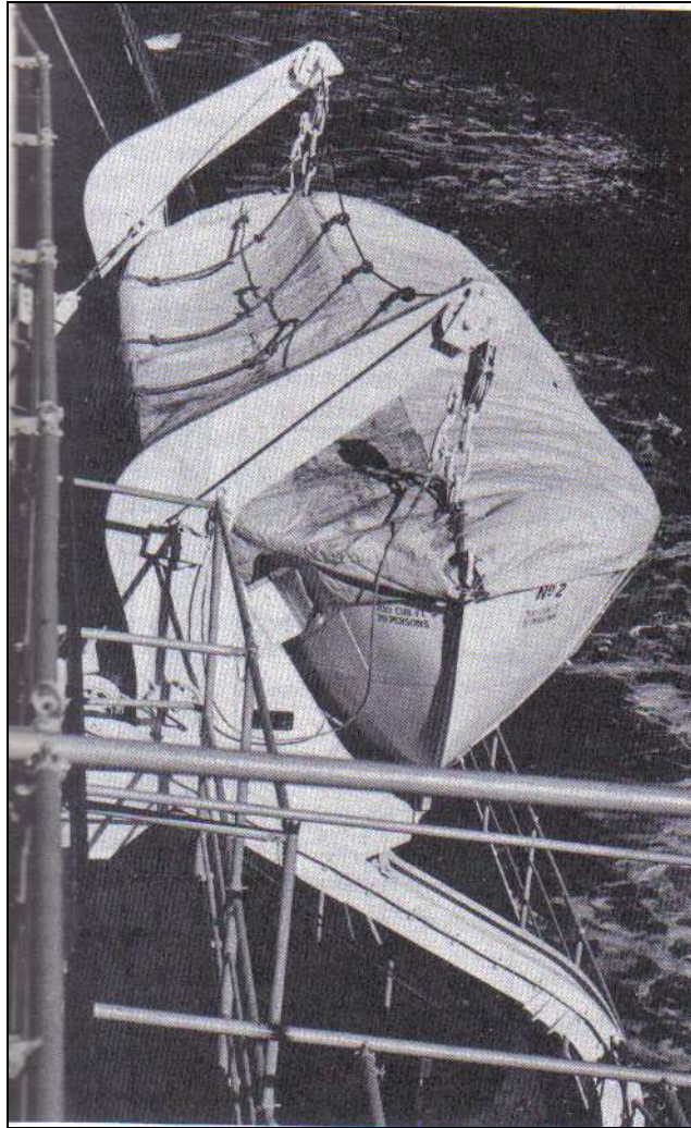
Fig. 5.26 – Example of a lifeboat installed on a gravity davits.
