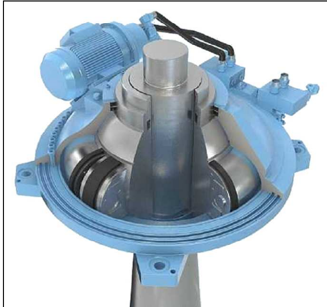
Fig. 3.38 – 3D cutaway of a spherical steering gear.
