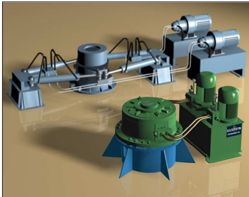
Fig. 3.37 – 3D view of ram versus rotary vane steering gear hydraulic systems.
