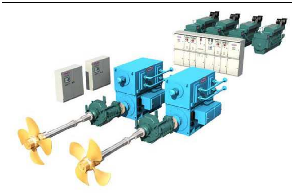
Fig. 2.105 – Fully electrical propulsion plant.
