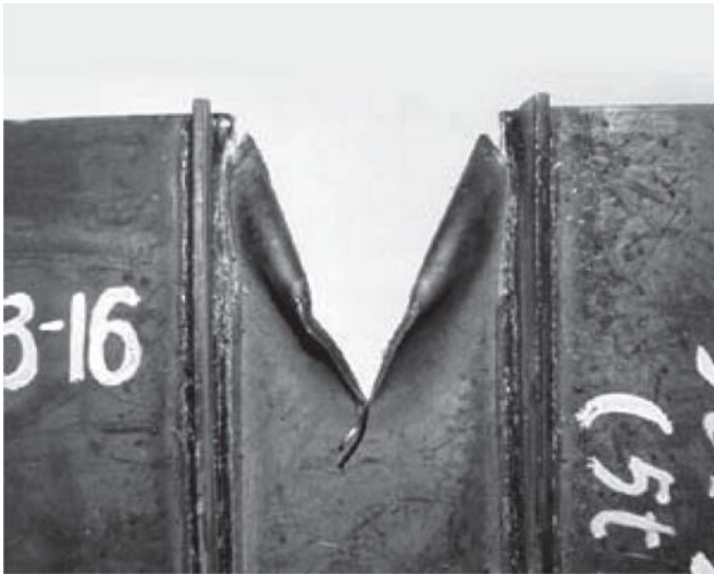
Fig. 143 Plate tearing of a tested specimen.
