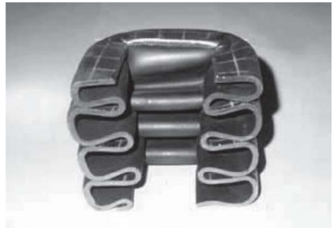
Fig. 150 A crushed tub under axial compressive load (forming of many folds) (Paik 2001).
