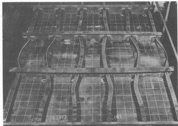
(b) INTERFRAME LATERAL-TORSIONAL BUCKLING (MODE 3)
