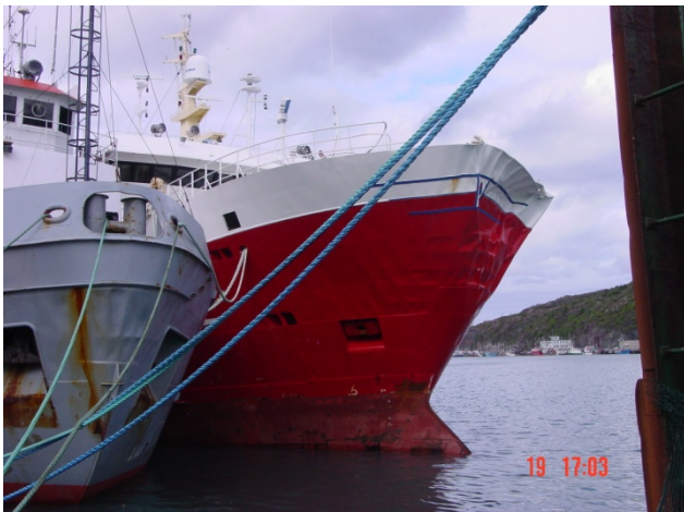
Local ice damage
