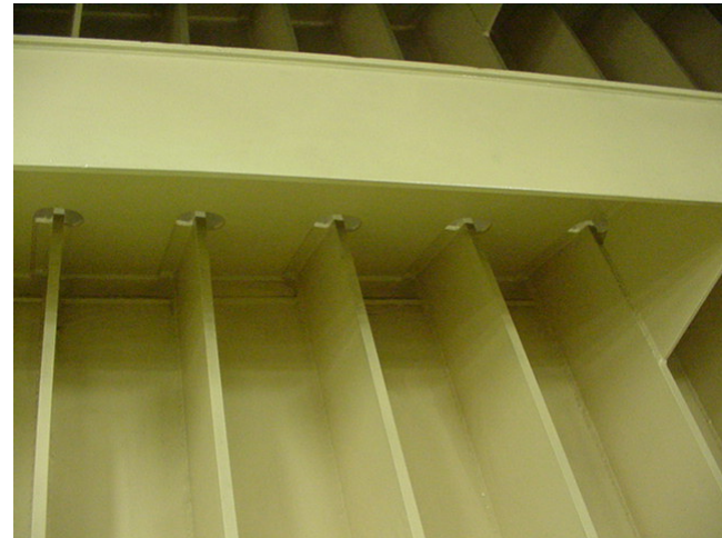
Transverse flat bar frames through stringer
