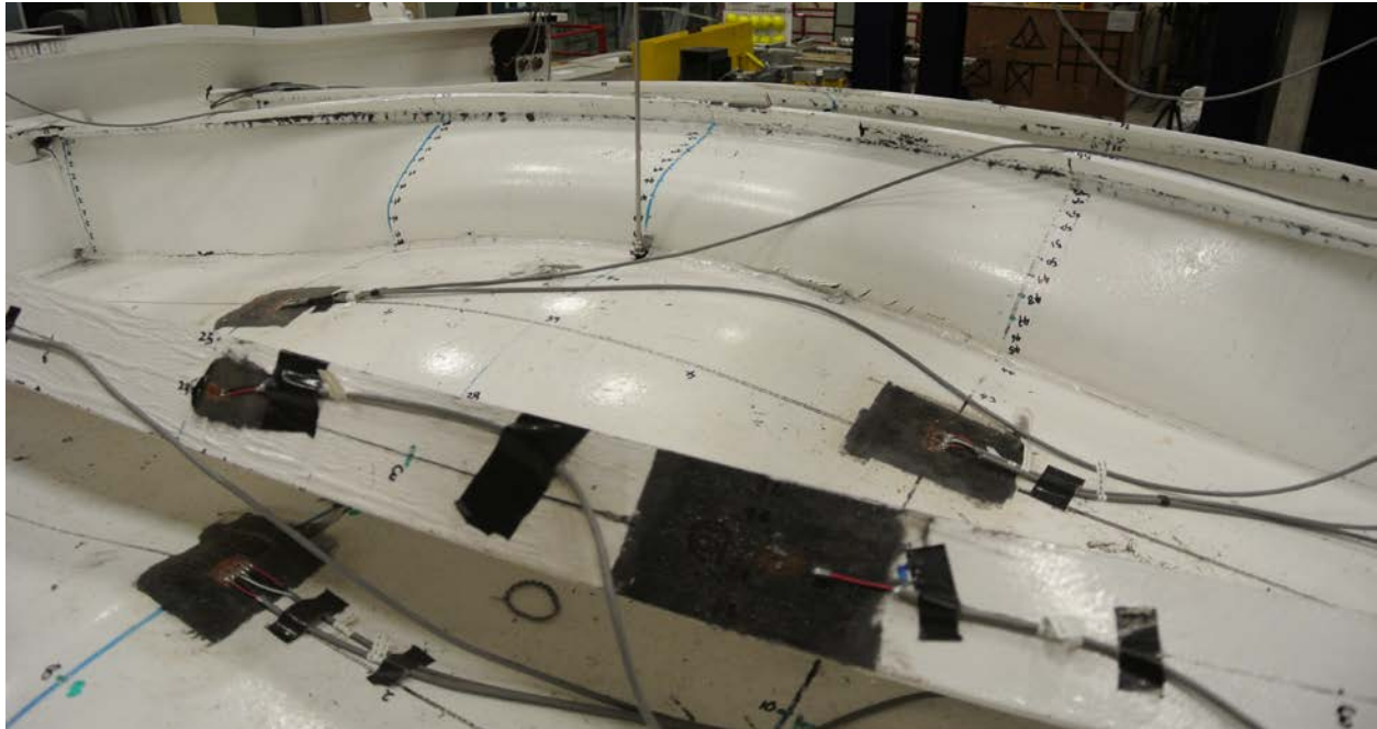
plastic frame response to ice load test
