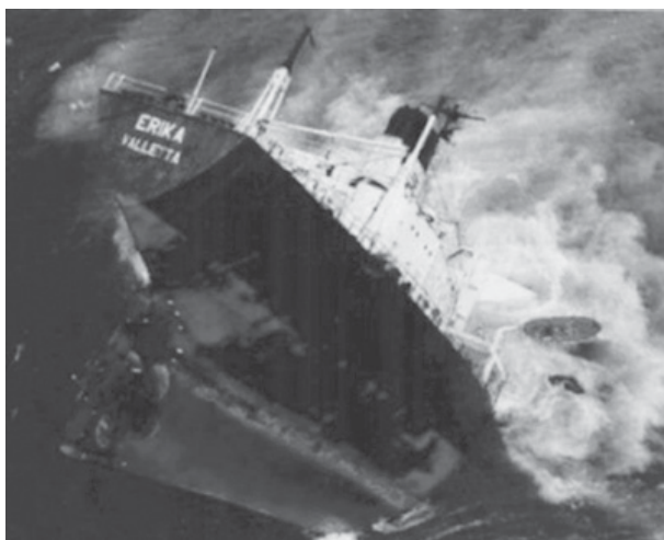
Figure 16.6 The back of the 24-year-old Erika broke in rough weather conditions.
