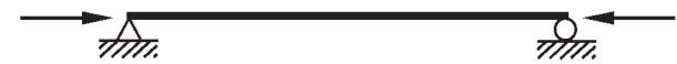
Figure 8.6b One-bay plate-stiffener combination model for a stiffened plate structure under uniaxial compression.
