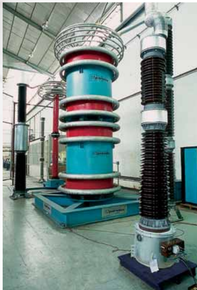
Routine tests of a 245 kV Capacitor Voltage Transformer.
