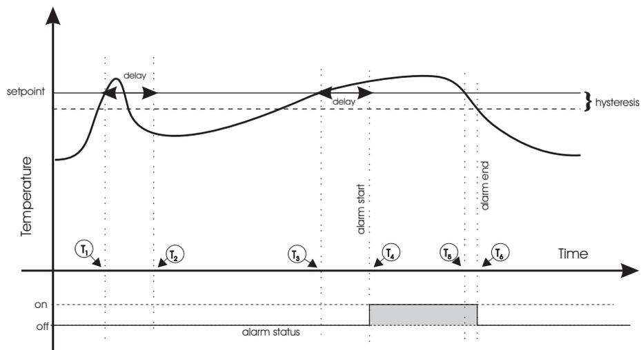
the set delay, at time  $T_4$ , the output channel is activated. At time  $T_5$  the curve representing temperature goes under the setpoint, but the alarm is de-activated at time  $T_6$  when it goes under the value of the setpoint minus hysteresis.
