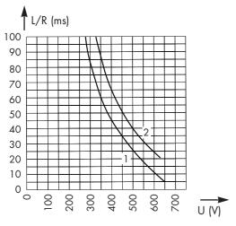
These curves indicate the permissible value of time constant L/R as a function of the D.C. working voltage.
