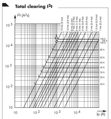
The flat curves show for each rated current the maximum values of total clearing I²t (I²t₁) as a function of a prospective current Ip. @ 690 V.  $\cos \varphi = 0.15$  (125-135 A @ 600 V. $\cos \varphi = 0.15$ )
