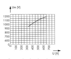
This curve indicate the peak ars voltage Um which may appear across the fuse terminals at working voltage U.
