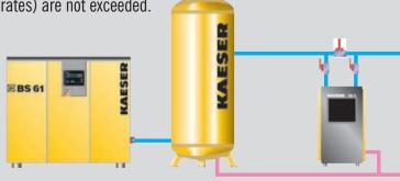
Reliable drainage at all condensate collecting points of the air system must be guaranteed. The best way of ensuring this is to use electronically controlled condensate drains
