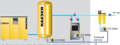
All collection points must be fitted with a reliable means of draining condensate. An electronic controlled, automatic drain unit is the best solution.
