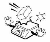
Grab on the bottom of the scale when moving. Do not hold by the platter.
